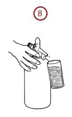
Remove the bulb holder and bulb from the thread. You will hear a short hiss.
