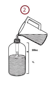
Insert the level tube into the bottle. You should hear and feel it click into place when the tube and top of the bottle are level. Fill the bottle until water spills over the top.
