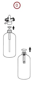
Use the enclosed tool to remove the level tube.
