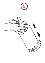
Place a CO2 bulb in the bulb holder and screw in onto the thread. You will hear gas enter the bottle; the siphon is now pressurized. Vigorously shake the Siphon several times.
